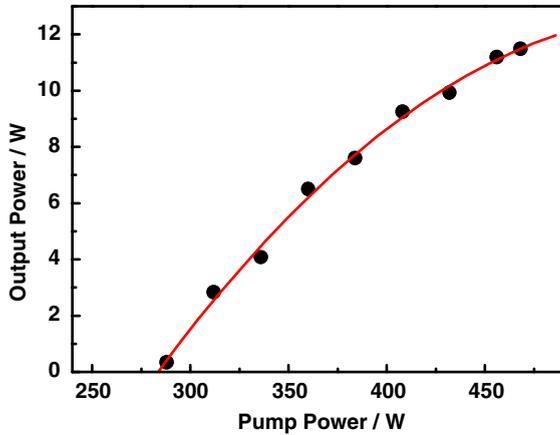
Fig. 3. The output power of red light at 659.5 nm versus pump power.
