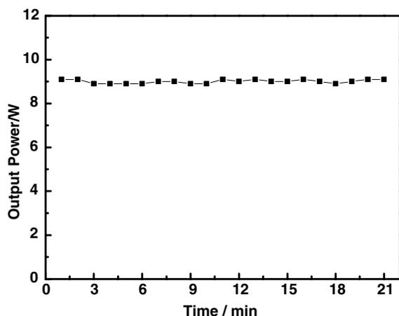
Fig. 5. Stability of the red output power at output power of 9 W. At the maximum output power of 11.5 W, the stability is about 10%.
