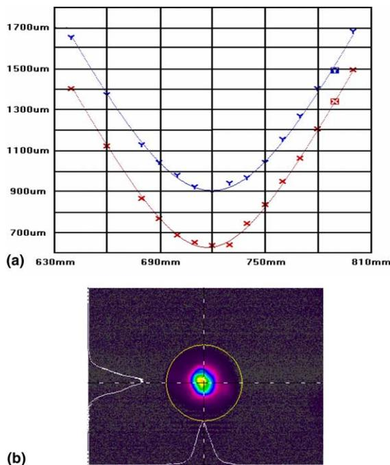
Fig. 7. The characterizations of beam quality of laser at maximum output power: (a) The measured beam radius with fitted curves for both transverse directions along the direction of propagation:  $X$ , the beam widths at  $x$ -direction;  $Y$ , the beam widths at  $y$ -direction directions. (b) Far-field intensity distribution of the beam.
