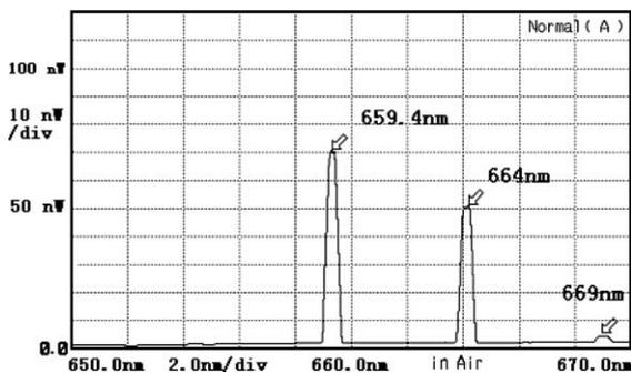
Fig. 4. The spectrum of the red beam under highest output power. Under lower pump power, the lights at 664 and 669 nm are ignorable than the one at 659.4 nm.
