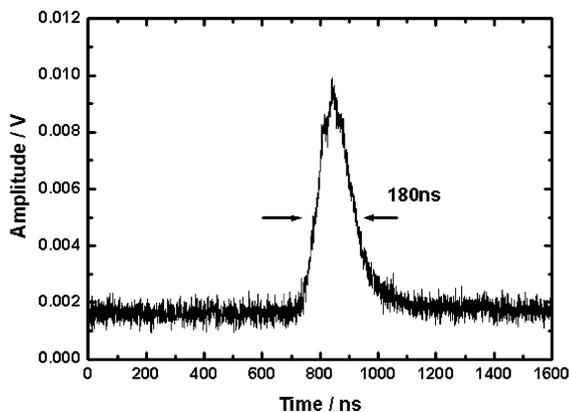
Fig. 6. The temporal profile of red beam.
