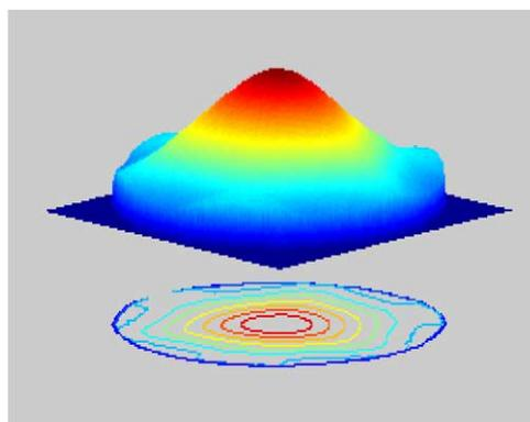
Fig. 2. Pump energy distribution within Nd:YAG rod. The pump energy distribution value is normalized in the upper figure. Each line represents a 12.5% change in intensity in the lower figure.
