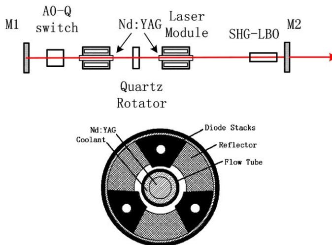
Fig. 1. The schematic drawings of the experimental arrangement: M1, M2, plane cavity mirror; AO-Q switch, acousto-optic Q switch.
